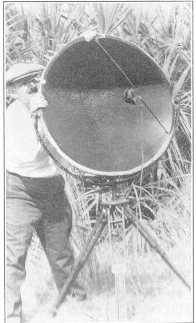
Parabolic microphone used in the field, from Albert R. Brand, "The 1935 Cornell-American Museum Ornithological Expedition," The Scientific Monthly 41.2 (August 1935): 189
